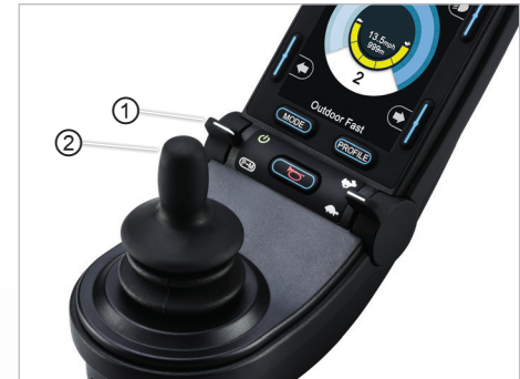
Fig. 66: Blocking the controls
